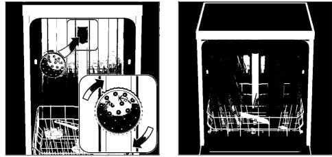
Large sheets or grilles and plates which have a diameter greater than 30 cm (gourmet plates, pasta plates, dinner plates) can be cleaned with the aid of the spray head. To do this, remove the top basket and insert the spray head as illustrated in the diagram.
