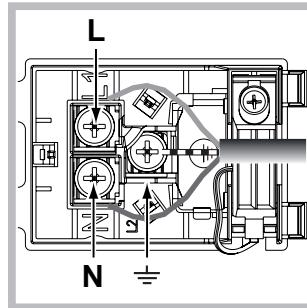
2. Install the power supply cable by loosening the cable clamp screw and the three wire contact screws L-N-GND.
